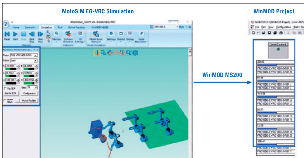
Illustration of the transmission of the axis values of a robot from MotoSIM EG-VRC (marked in red on the left) and the values transmitted via the WinMOD MS200 plug-in (marked in red on the right). The axis values on the WinMOD page correspond to the axis values of robots programmed offline.
