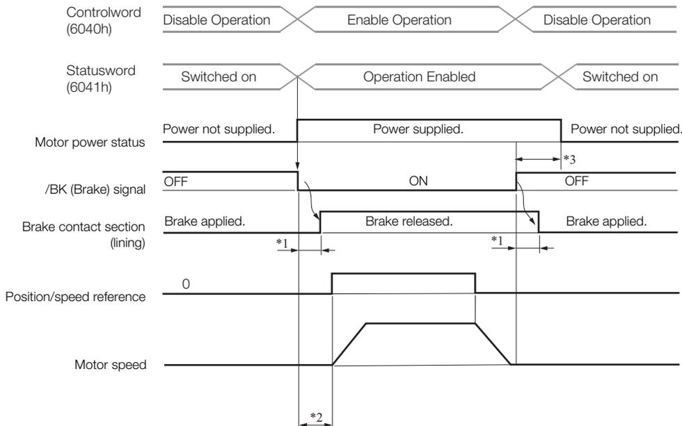
\*1. Rotary Servomotors: The brake delay times for Servomotors with Holding Brakes are given in the following table. The operation delay times in the following table are examples for when the power supply is switched on the DC side. You must evaluate the actual brake delay times on the actual equipment before using the application.
