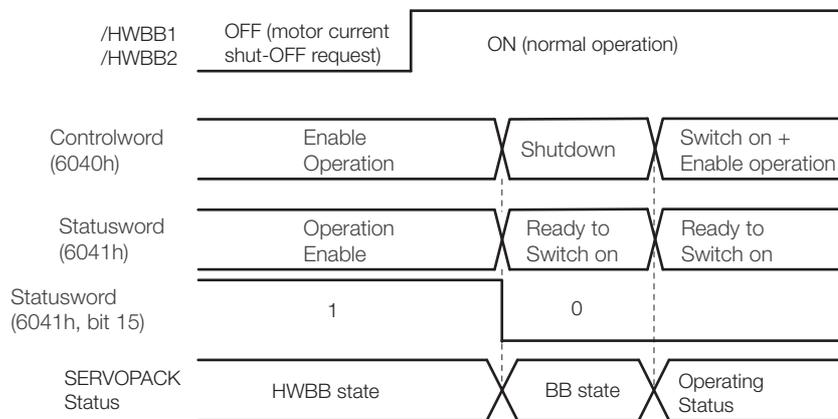
Note: If the SERVOPACK is placed in the BB state while the main circuit power supply is OFF, the HWBB state will be maintained until the Shutdown command is received.
