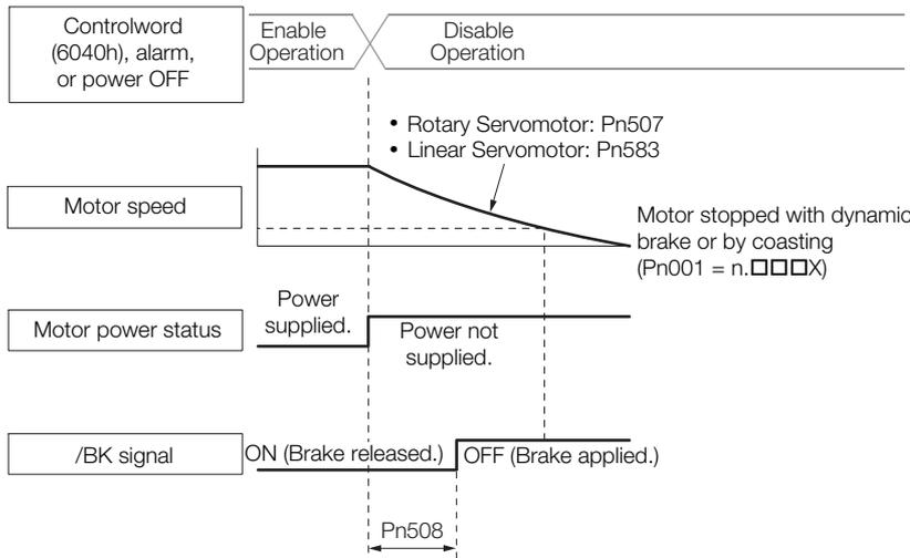
The Servomotor will be limited to its maximum speed even if the brake reference output speed level (Rotary Servomotor: Pn507, Linear Servomotor: Pn583) is higher than the maximum speed.
