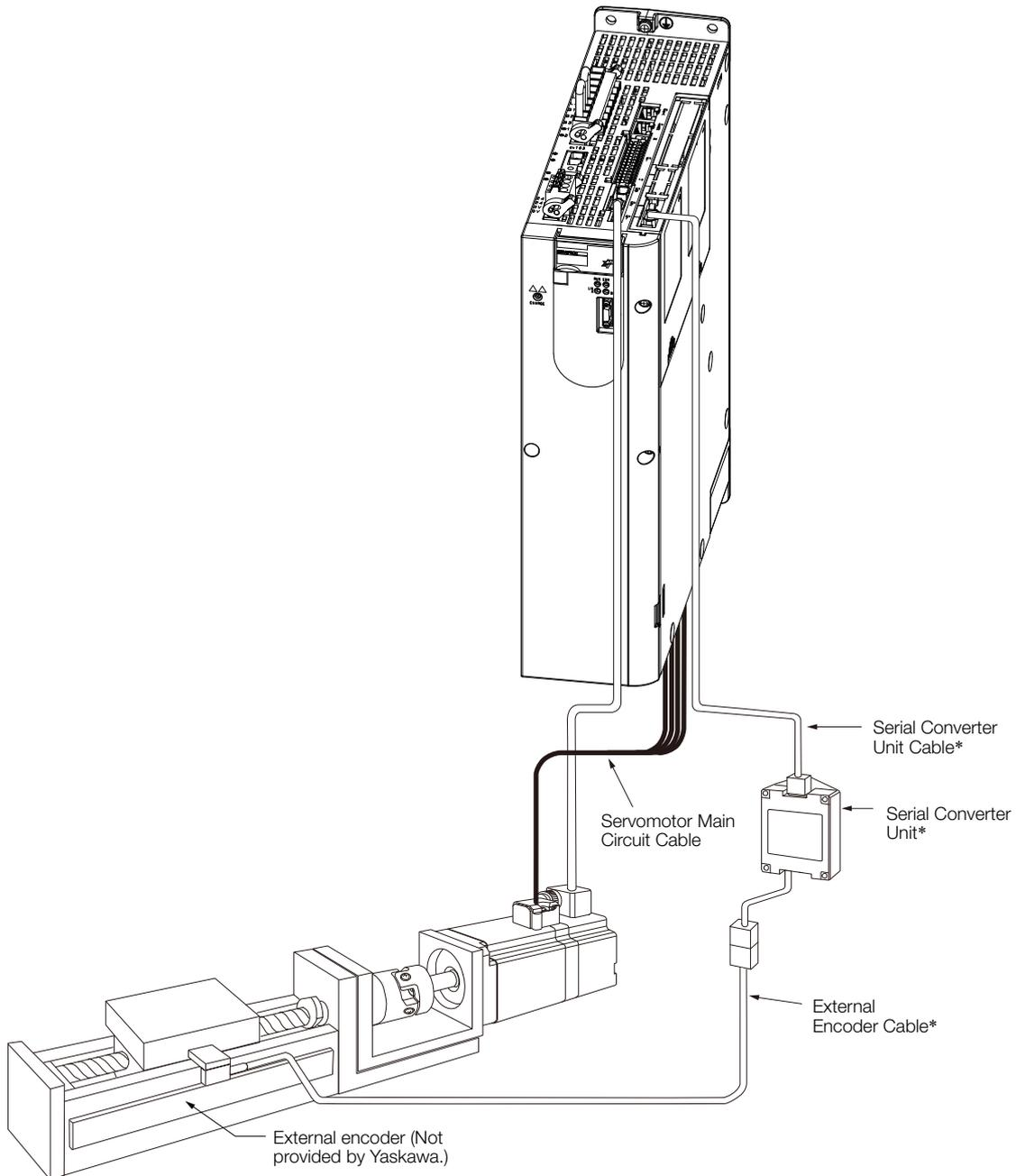
\* The connected devices and cables depend on the type of external linear encoder that is used.
