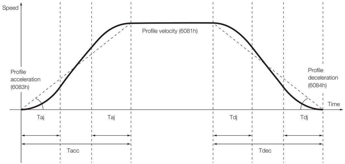
Acceleration time:  $T_{acc} = \frac{\text{Profile velocity (6081h)}}{\text{Profile acceleration (6083h)}}$
