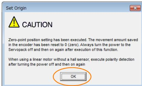
7. Turn the power supply to the SERVOPACK OFF and ON again.
