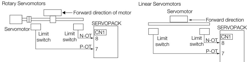
Using the overtravel function is not necessary for rotating applications such as rotary tables and conveyors. No wiring for overtravel input signals is required.
