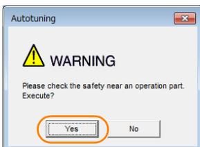
Tuning will be executed. Vibration that occurs during tuning will be detected automatically and suitable settings will be made for that vibration. When the settings have been completed, the indicators for the functions that were used will light at the lower left of the dialog box.
