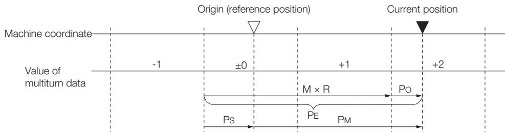
The current position  $P_M$  in the machine coordinate system is calculated as follows:
