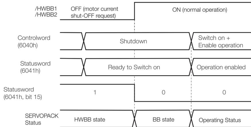
If the /HWBB1 and /HWBB2 signals are OFF and the Servo ON command (Enable Operation command) is received, the HWBB state will be maintained even after the /HWBB1 and /HWBB2 signals are turned ON.
