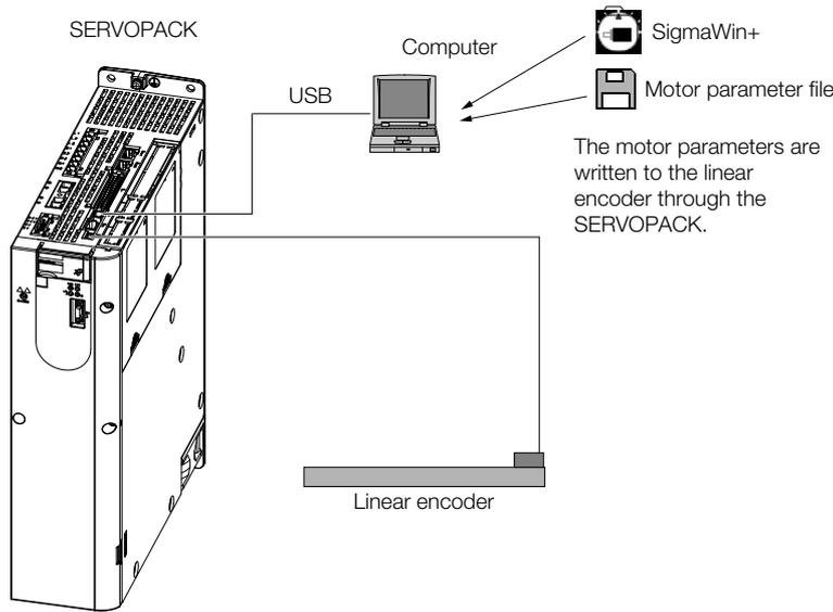
**Important** Serial number information is not included in the motor parameters. You cannot use the monitor functions of the SERVOPACK to monitor the serial number. If you attempt to monitor the serial number, \*\*\*\*\* will be displayed.
