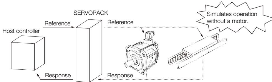
Use Pn00C = n.□□□X to enable or disable the test without a motor.
