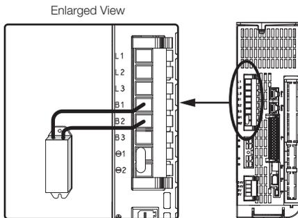
3. Set Pn600 (Regenerative Resistor Capacity) and Pn603 (Regenerative Resistor Resistance). Refer to the following section for details on the settings.
