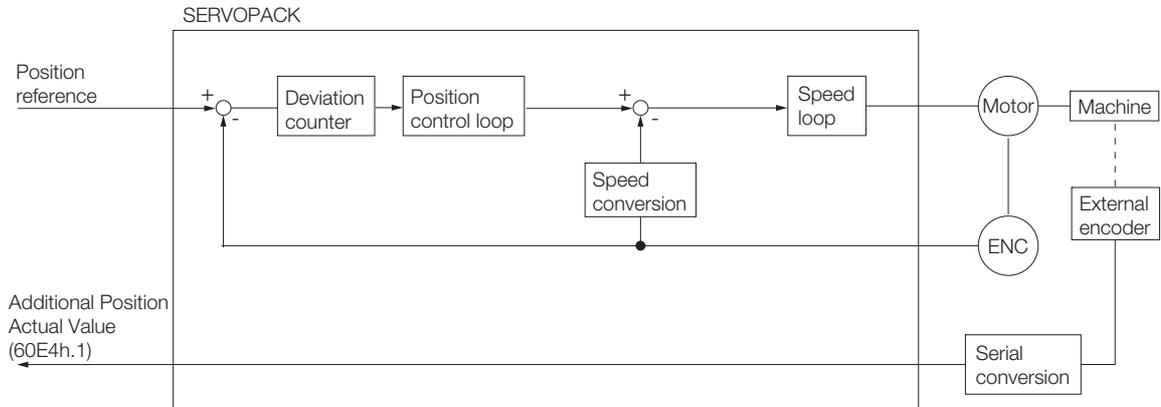
The following block diagram shows monitoring an external encoder in the Profile Position Mode.
