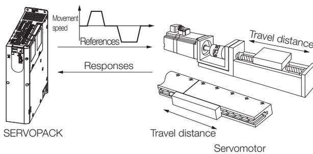
Note: Execute autotuning without a host reference after jogging to a position that ensures a suitable range of motion.
