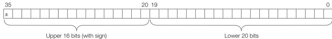
When the SERVOPACK sends the position data, it sends the upper 16-bit data (with sign) separately from the lower 20-bit data.
