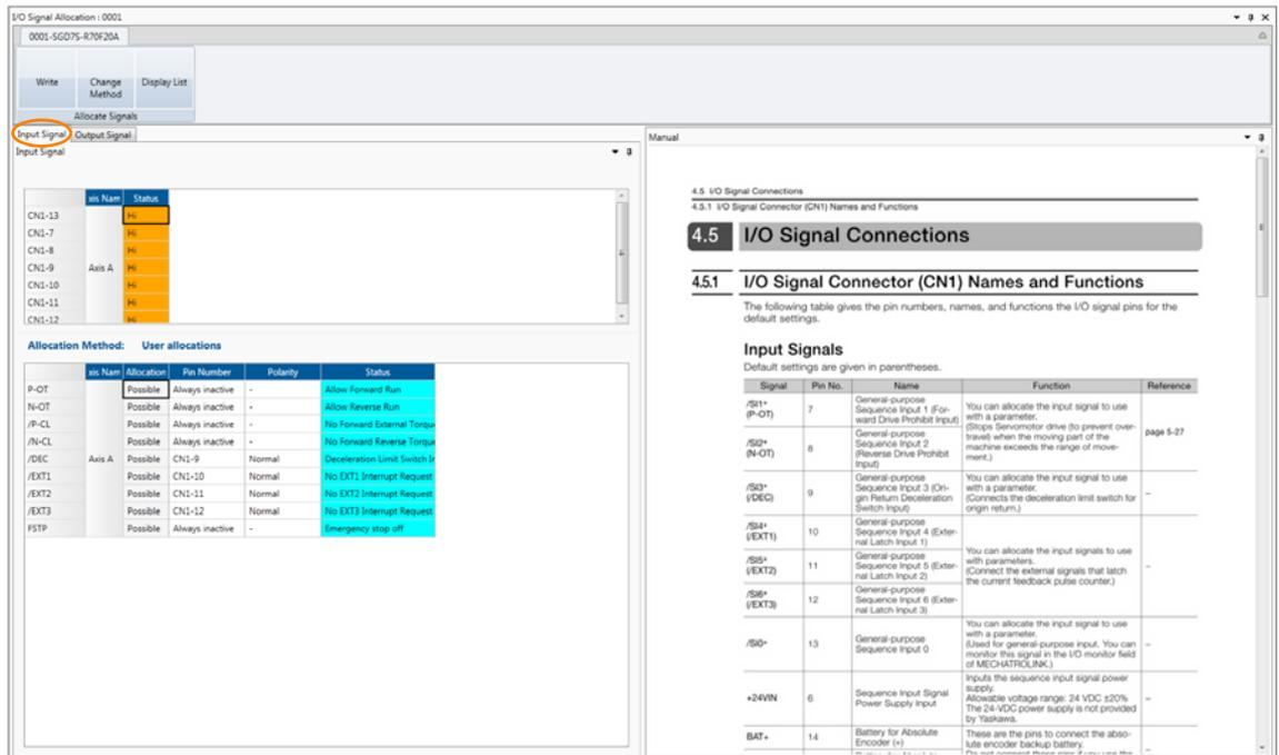
The screenshot shows the 'I/O Signal Allocation : 0001' window for device '0001-SGD7S-R70F2DA'. The 'Input Signal' tab is selected, showing a table of input signals for Axis A. The 'Manual' pane on the right displays the '4.5 I/O Signal Connections' section, specifically '4.5.1 I/O Signal Connector (CN1) Names and Functions'. It includes a table of input signals with columns for Signal, Pin No., Name, Function, and Reference.
