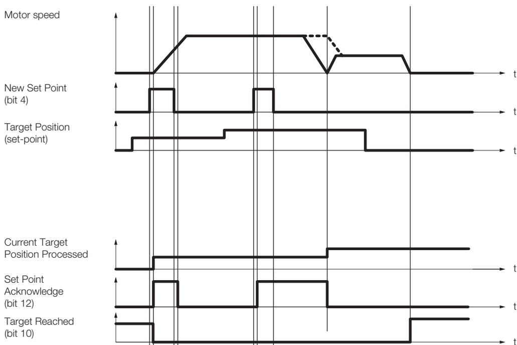
◆ **SPOSING (S-curve Acceleration/Deceleration Positioning)**
