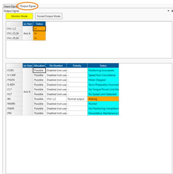
The screenshot shows the 'Output Signal' tab selected in the 'I/O Signal Allocation' window. It displays a table of output signals for Axis A, including their names, allocation status, pin numbers, polarities, and current status.
