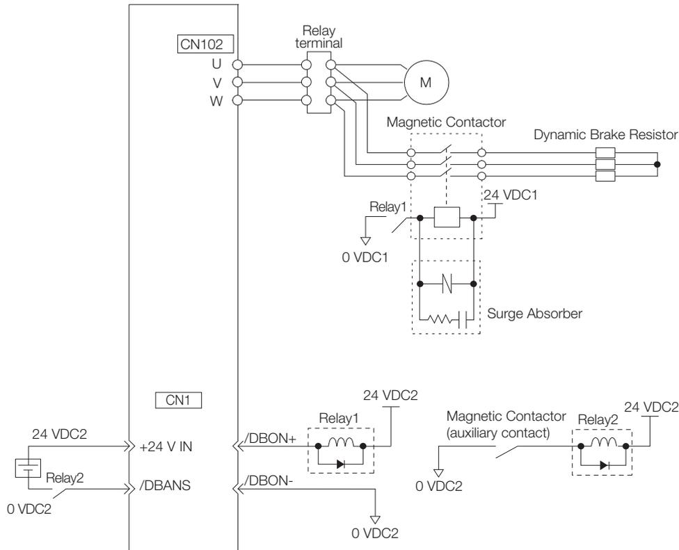
Note: 1. Separate the 24-VDC power supply for the Magnetic Contactor from the power supply for the I/O signals (CN1). If the same power supply is used, the I/O signals may malfunction.
