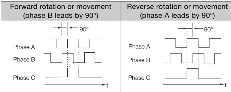
Note: The pulse width of encoder phase C depends on the setting of Pn212 (Number of Encoder Output Pulses) or Pn281 (Encoder Output Resolution). It is the same as the width of phase A. Even for Pn000 = n.□□□1 (reverse operation), the output phase form is the same as shown above.
