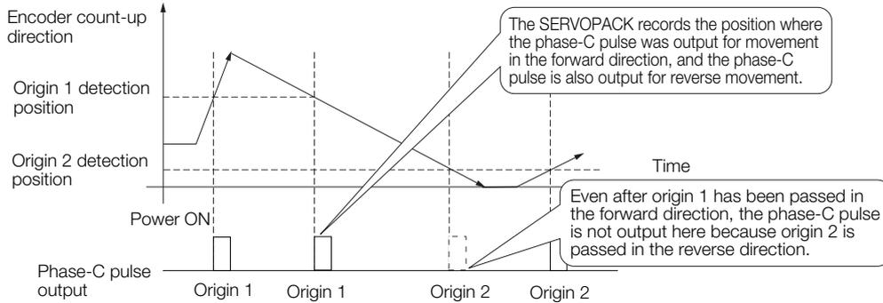
■ When Using a Linear Encoder with Multiple Origins and First Passing the Origin Position in the Reverse Direction after Turning ON the Power Supply
