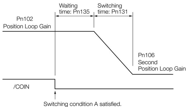
**Information** You can use gain switching for either PI control or I-P control (Pn10B = n.□□0□ or □□1□).
