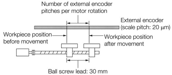
If the external encoder is connected directly to the Servomotor, the setting will be 1,500 (30 mm/0.02 mm = 1,500).
