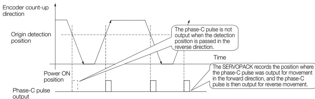
■ When Using a Linear Encoder with Multiple Origins and First Passing the Origin Position in the Forward Direction and Returning after Turning ON the Power Supply
