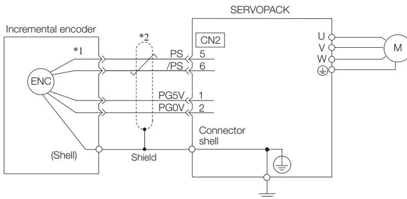
\*1. The incremental encoder pin numbers for wiring the connector depend on the Servomotor that you use.
