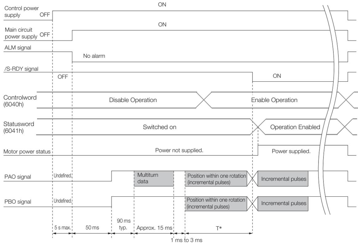
\* The pulse output time T for the position of the absolute encoder within one rotation depends on the setting of Pn212 (Number of Encoder Output Pulses). Refer to the following table.
