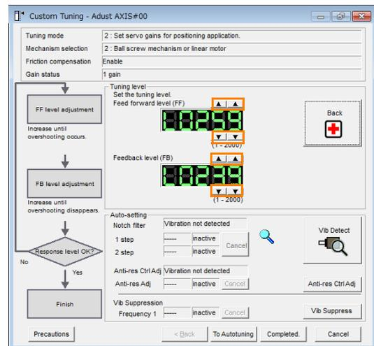
**Information** The new feedforward level will not be used until the positioning completed signal is output.
