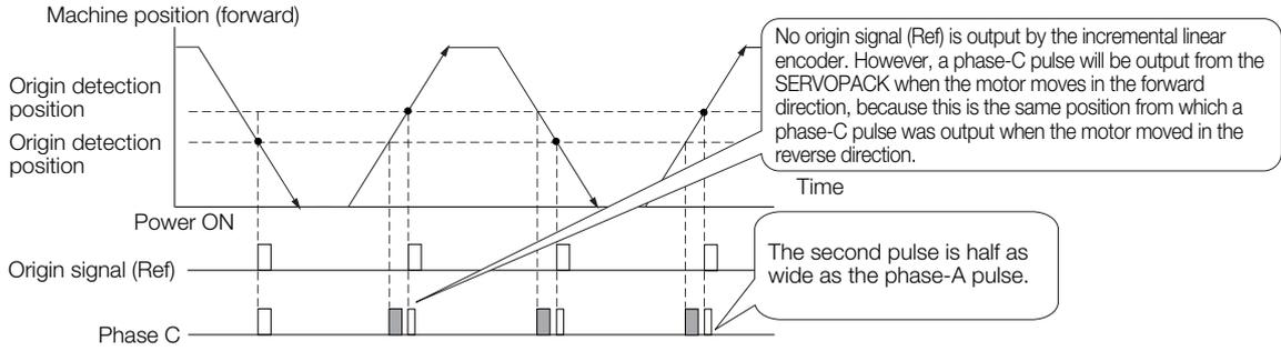
◆ Precautions When Using a Linear Incremental Encoder from Magnescale Co., Ltd.
