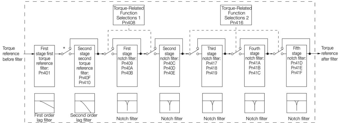
\* The second stage second torque reference filter is disabled when Pn40F is set to 5,000 (default setting) and it is enabled when Pn40F is set to a value lower than 5,000.
