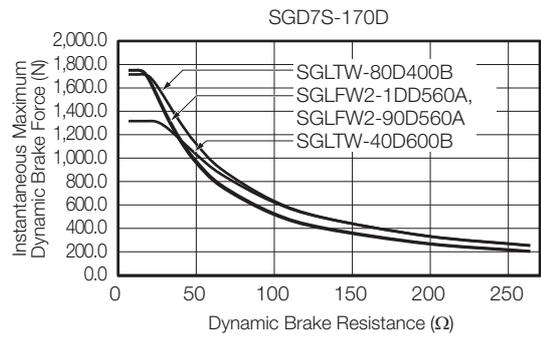
◆ Energy Consumption of the Dynamic Brake Resistor
