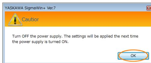
7. Turn the power supply to the SERVOPACK OFF and ON again after the parameter settings have been initialized.
