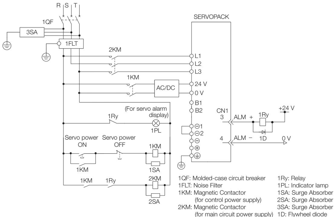
4.3 Wiring the Power Supply to the SERVOPACK
