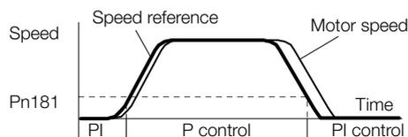
■ Using the Acceleration as the Mode Switching Condition
