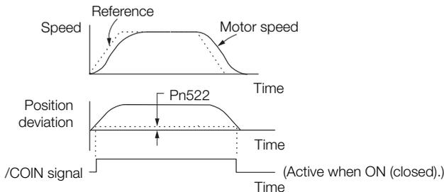
Note: If the parameter is set to a value that is too large, the /COIN signal may be output when the position deviation is low during a low-speed operation. If that occurs, reduce the setting until the signal is no longer output.
