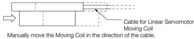
5. If the feedback pulse counter counts up, set a phase-A lead as a phase sequence of U, V, and W (Pn080 = n.□□0□).
