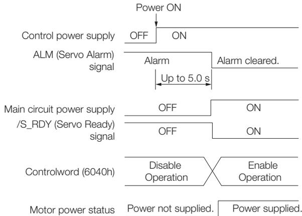
**Information** If the servo ON state cannot be achieved by inputting the Servo ON command (Enable Operation command), the /S\_RDY signal is not ON. Check the status of the /S\_RDY signal. Refer to the following section for details.
