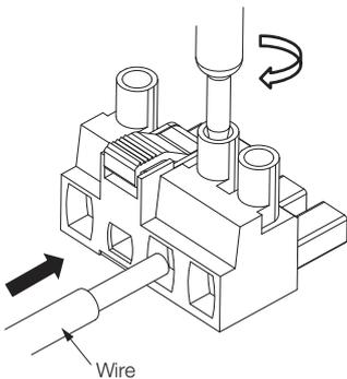
6. Connect the Dynamic Brake Resistor to the D1 and D2 terminals on the SERVOPACK.
