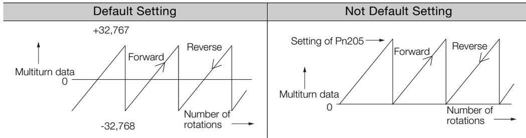
**Information** When the encoder is set to be used as a single-turn absolute encoder (Pn002 = n.□2□□), the multiturn data will always be zero. It is not necessary to reset the absolute encoder. Also, an alarm related to the absolute encoder (A.810 or A.820) will not occur.
