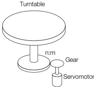
Because the turntable moves in only one direction, the upper limit to the number of rotations that can be counted by an absolute encoder will eventually be exceeded.
