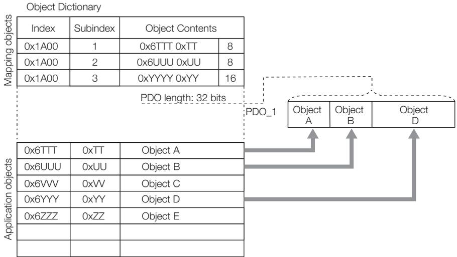
In addition to the above PDO mappings, PDOs have to be assigned to the Sync Managers to exchange EtherCAT process data.
