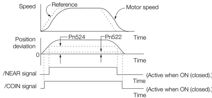
Note: Normally, set Pn524 to a value that is larger than the setting of Pn522 (Positioning Completed Width).
