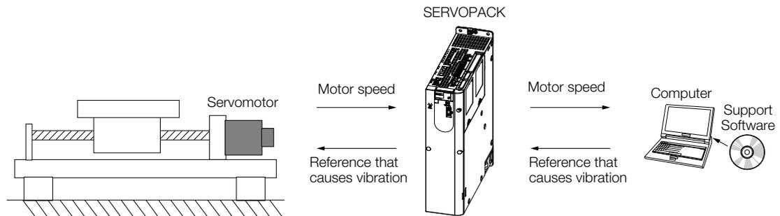
The Servomotor is used to cause machine vibration and then the speed frequency characteristics for the motor torque are measured. The measured frequency characteristics can be used to determine the machine resonance.
